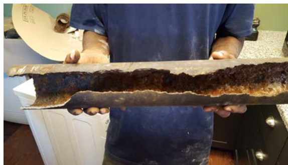
Examples of Cast Iron Piping Replaced at Pointe Towers
