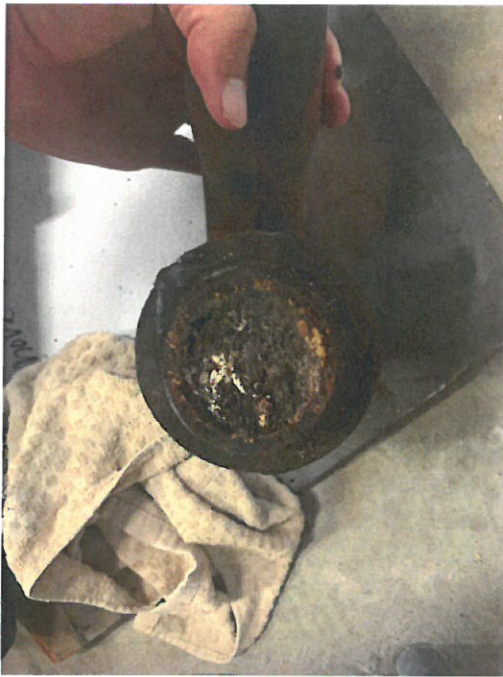
P-Trap Blockage of Unit 4S
