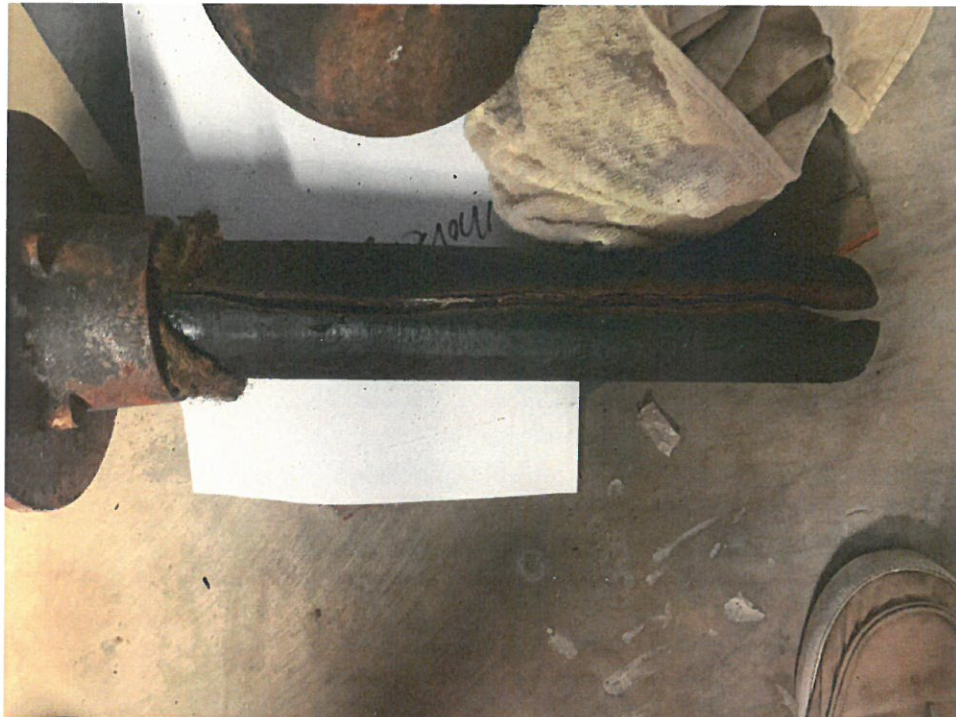
Cracked Pipe from Shower Drain of Unit 4S
